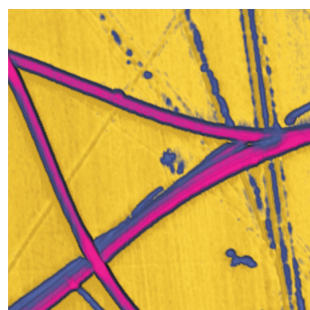
Self-assembled diphenylalanine peptide nanotubes: simultaneous topography, adhesion, d^2C/dZ^2 and in-plane piezoresponse phase (direction of polarization) measurements obtained by HD mode, 8x8 \mu\text{m}
