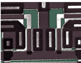
Topography of microchip, 70x46 \mu\text{m}
