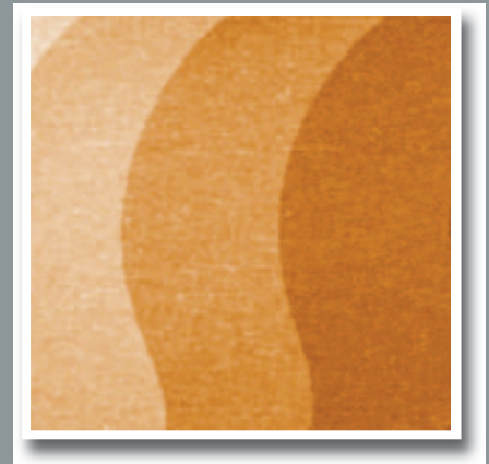
Silicon Test Echeloned Pattern STEPP. Monatomic step image with closed-loop on. Step height 0.31 nm. Scan size 7x7 μm
